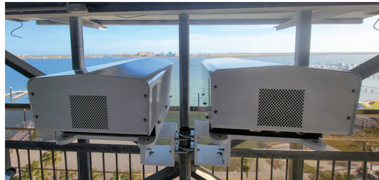
The WAV Surveillance System can generate a 90 degree field of view high-resolution image at 1 Hz that is then processed for detection and tracking.
