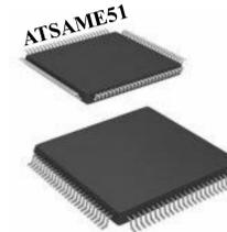
To meet the demands of each of the subsystems, the ATSAME51 uses 100 pins in order to effectively operate the entire testbed. Every command from the computer is sent to the microcontroller which dictates which sequence or process is needed to start.
