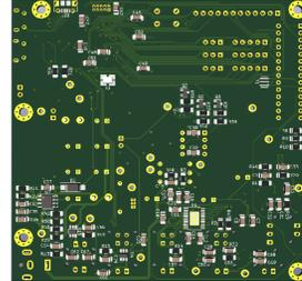
The board is powered by a 19.8V laptop power adapter which is convenient for transport and user friendly. The middle two layers are for 3.3V and GND, allowing for cleaner tracing across the entire board and giving room for a compact design. In the case of failure, an ATmega is placed on the board to allow for testing and running the subsystems, independent of the main controller.
