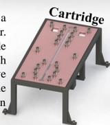
The TEC module is a Thermo-Electric Cooler, that is in between a plate of aluminum, that aids in dispersing heat into the cartridge. A heat sink aids in the dissipation of heat from the assembly. The TEC assembly allows for cyclic heating and cooling of the biological liquid in the cartridge and conducts the biological process of thermocycling. This assembly also includes an RTD sensor that measures the changing temperature of the system.
