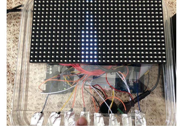
**Keyboard/Tune Generator** – When activating the capacitive touch, the Arduino then plays a certain tune or frequency, each at a different pitch from the others.
