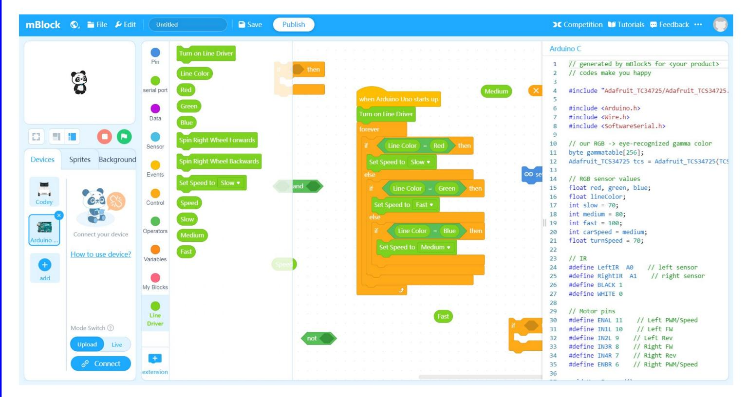
**The App:** This robot will be totally controlled by the kids at MakerKids. It utilizes mBlock, an Arduino-compatible version of Scratch, to incorporate a drag and drop style of coding the robot. We provide custom blocks that handle all of the heavy lifting, so the kids can design a course for the robot to drive on and learn how to code in a high level block design.
