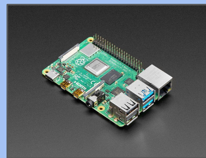
Raspberry Pi 4 Host web server for web application (Node JS)
