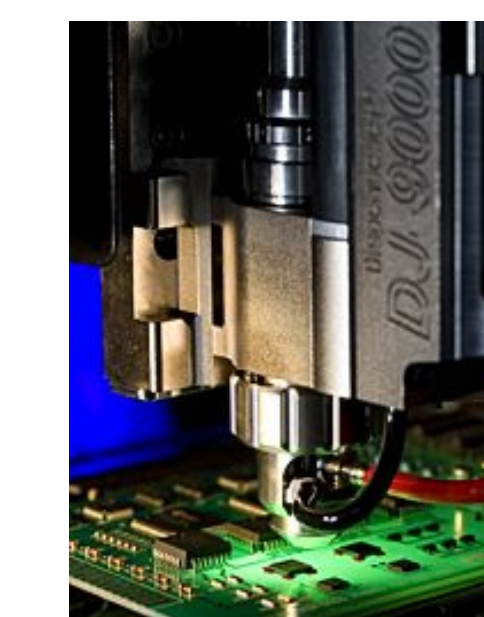
4. Vantage dispenses adhesive onto PCB
