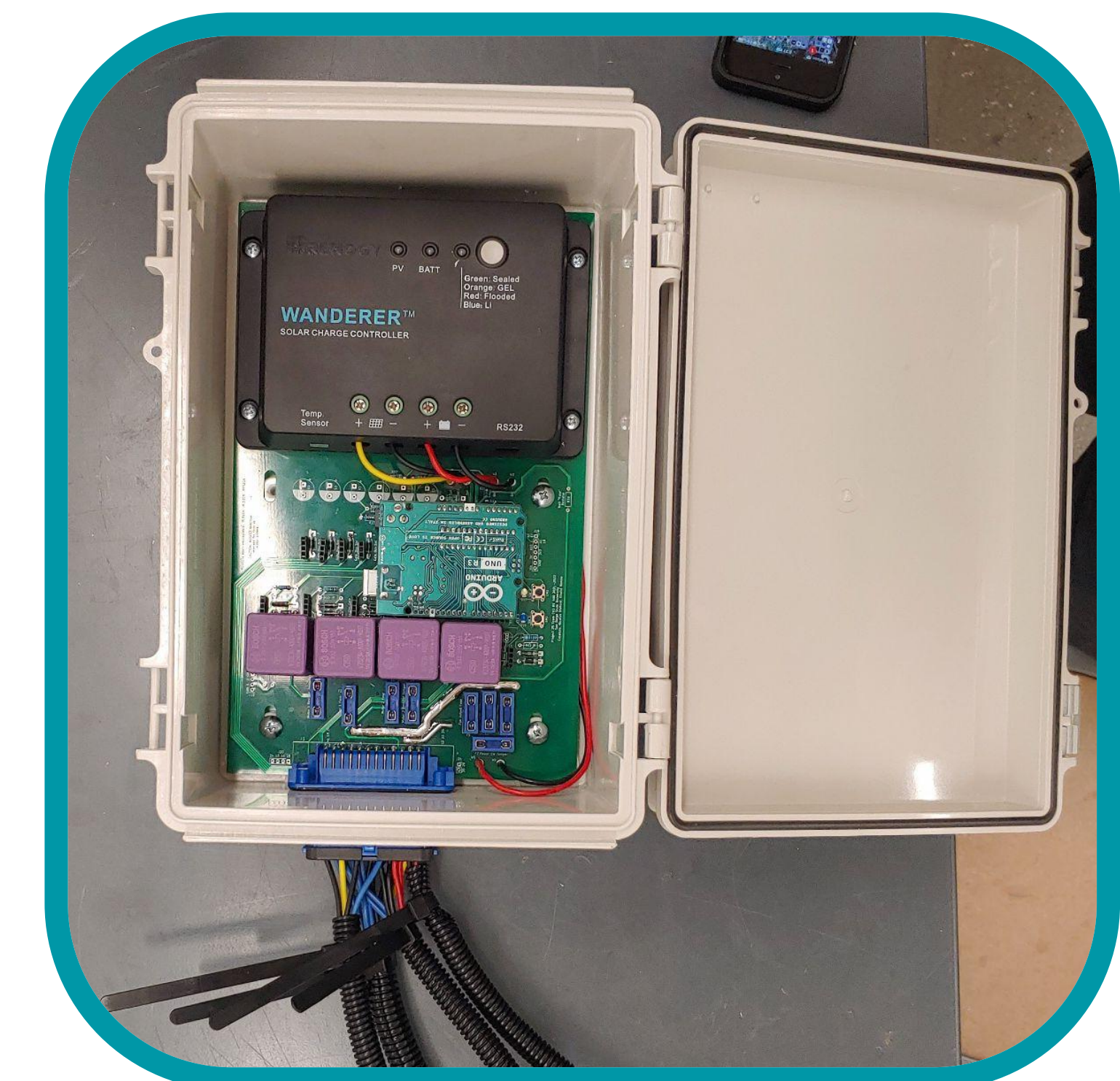
Electrical Components Enclosure: Solar Charge Controller and PCB Board
