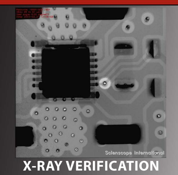
X-Ray analysis of the 12V buck converter IC. This test confirmed that the solder joints were formed properly.
