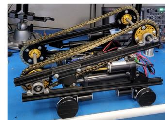
**Small-scale prototype:** Used for early development and testing of electronics and controls code.
