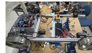
**Electronics Integration:** Mounting all electrical components and ensuring that procured items, custom PCBs, and code all work together reliably and with the desired behaviors.
