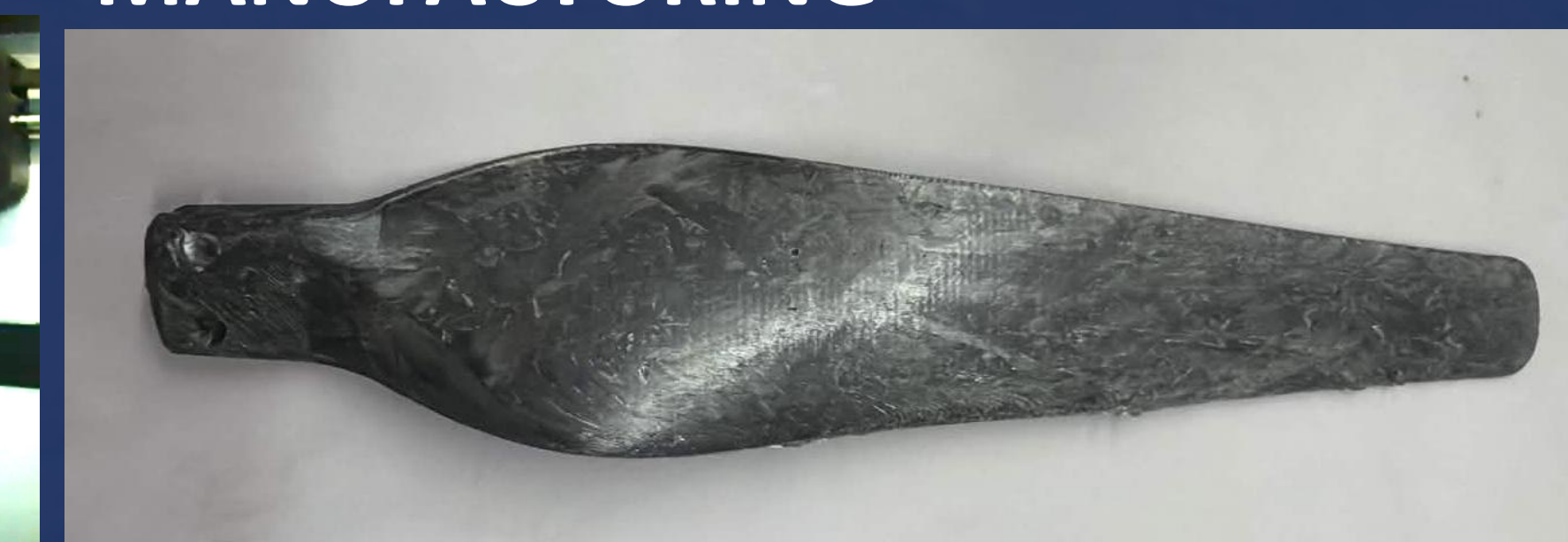
3D Printing Propellers (Left) and Carbon Fiber Forged Propeller (Right)
