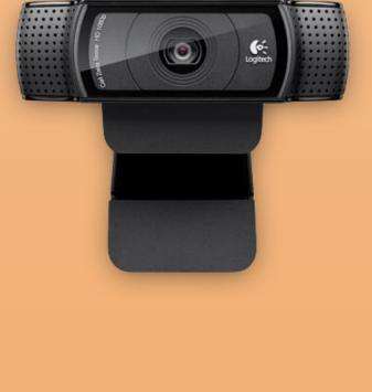
A 1080P camera which includes built in H.264 video compression. Used with TX2's H.264 decoder, we achieve 30 FPS while running YoloV3 Tiny weights.
