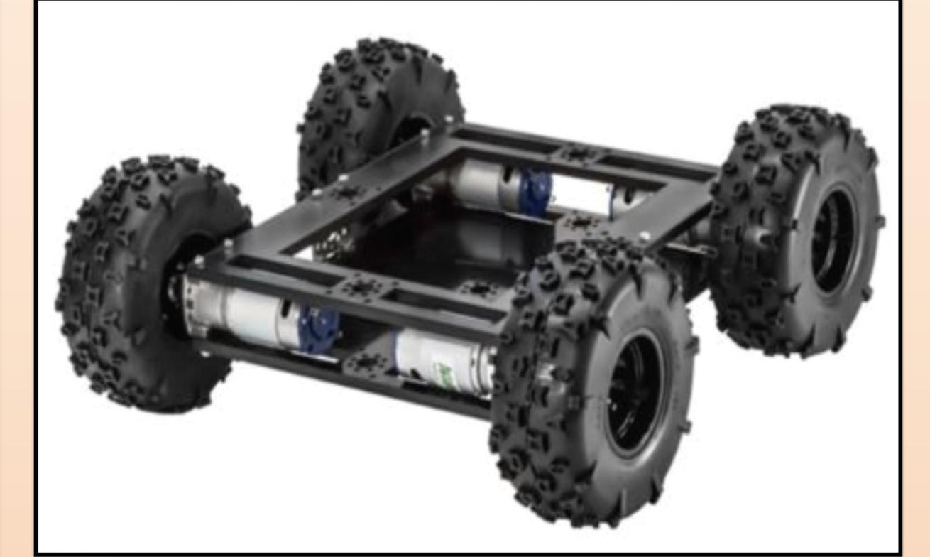
The Smile-Mobile consists of a vehicle frame with batteries and boards mounted internally and a camera mounted on the external frame.
