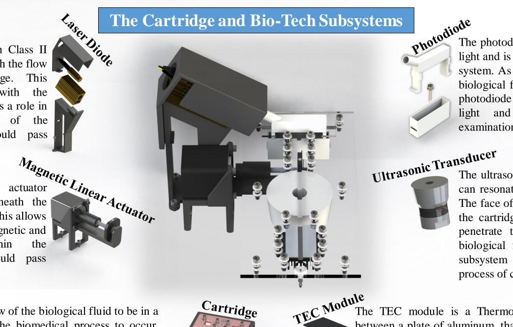
The laser diode is a green Class II laser oriented to pass through the flow path within the cartridge. This subsystem corresponds with the photodiode system and plays a role in the optical examination of the biological fluid that would pass through the cartridge.
