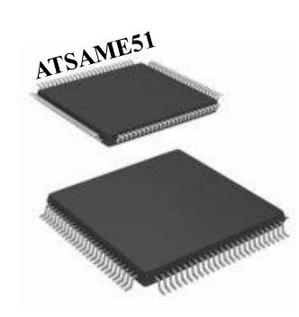
To meet the demands of each of the subsystems, the ATSAME51 uses 100 pins in order to effectively operate the entire testbed. Every command from the computer is sent to the microcontroller which dictates which sequence or process is needed to start.
