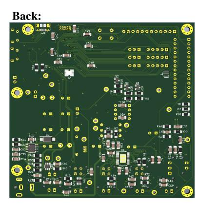
The PCB makes use of both sides of the board, using both through hole and surface mount components. The use of both allow for a reduced size as well as the capability to handle higher voltages and currents where necessary. Using vertical Molex connectors, which are all positioned at the bottom of the board, allows for easy access and adjustment as well as a quick disassembly.
