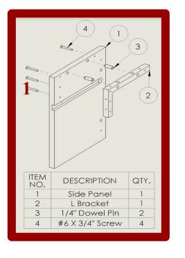
2. Cabinet panels have pre-drilled pilot holes and contain dowel pins to properly to guide the 1" screws.
