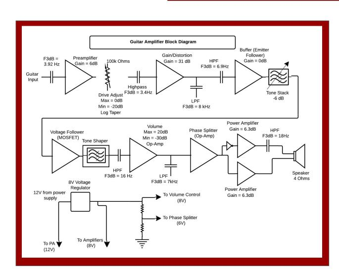
The design follows the general composition of a guitar amplifier with the following stages: preamplification, distortion, tone adjust, volume, gain, and power amplification
