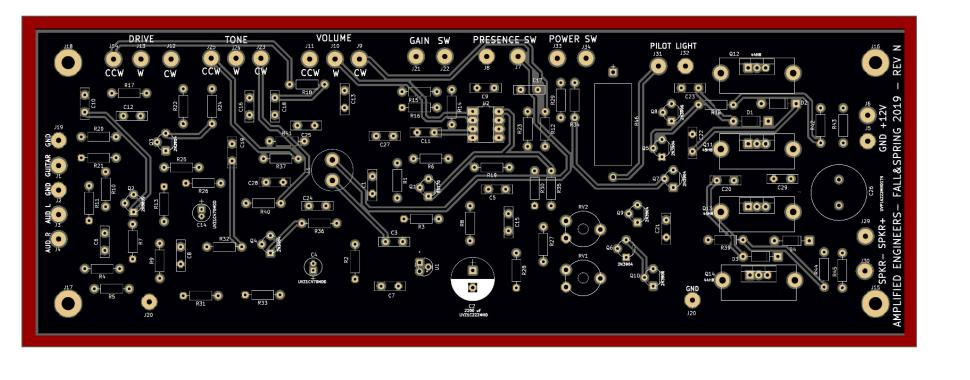
The PCB layout was designed in conjunction with the ME team in order to ensure a proper fit with the final cabinet design. Some of the components are rather tall and could have resulted in collision without careful planning.
