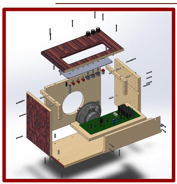
The final design was centered around manufacturability, ease of assembly, portability, aesthetic appearance, and price point. Designed with the assembly process in mind, the kit caters towards high school students with limited mechanical experience. The completed amplifier is constructed of ½" baltic birch plywood wrapped in Tolex. It measures 12" x 10" x 7" and weighs under 15 lbs.
