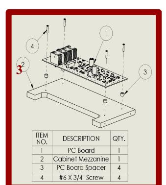
The mezzanine, complete with the PCB mounted and control components connected, slides into the grooves routed on the side panels. Next, the top panel is secured to the brackets with dowel pins. Finally, the interface components are inserted into the specified holes and secured from the top.
