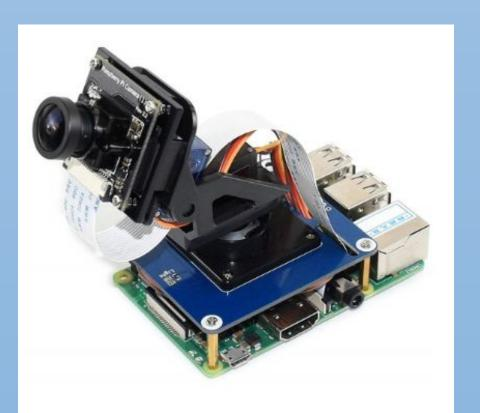
Raspberry Pi Camera Object detection system that identifies wildlife
