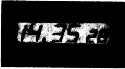
Fig. 2. Display operated in the reflection mode between crossed polarizers with 1.3-V rms 50-Hz square-wave excitation.
